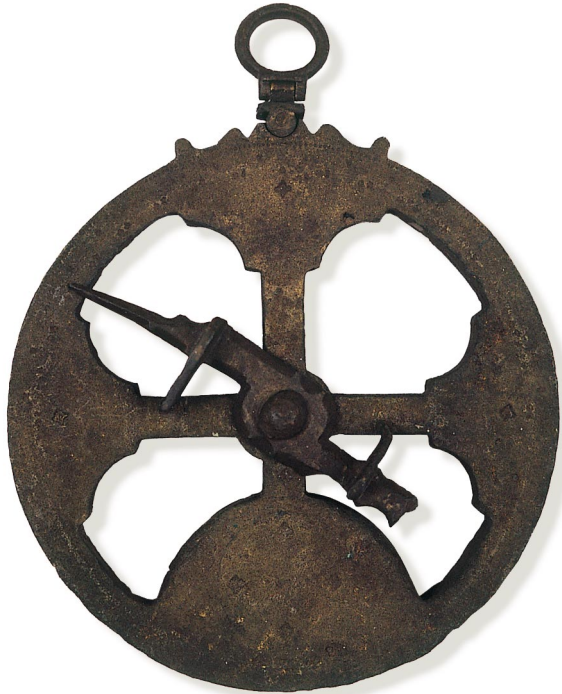
The Astrolabe that the Portuguese navigators used on board ship to calculate the height of the Sun throughout the day.
